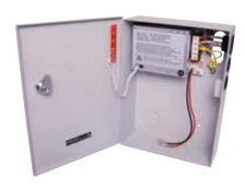
A complete 12V DC power supply and battery backup unit. When operating from 240V, it charges the internal battery (available separately) and powers the connected load (max 5A). When mains fails, the load is powered from the battery. Output short circuit protection, current limiting and over voltage protection. Low voltage cutoff @ 10.8V. Ideal for alarm backup use. Indoor use only. Includes power lead.
