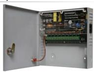
Designed for powering up to nine 12V DC powered CCTV cameras. Each output is individually fused and can be set on or off via internal jumpers. Outputs are protected to prevent damaging spikes and surges. Screw terminals are provided for each circuit. Output current limiting and over voltage protection included. Overall total continuous load is 7.5A with a peak current of 10A. Includes power lead. Indoor use only.
