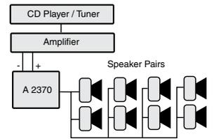
Designed for installations using several pairs of 8Ω speakers connected to one amplifier. Adjustable impedance protection allows multiple pairs of speakers to be connected without overloading the amplifier. Each pair is wired back individually to the transformer. Accepts up to 4 pairs of speakers totalling 150W, and can be placed in the ceiling space or behind the amplifier. Plug in terminals simplify installation.
